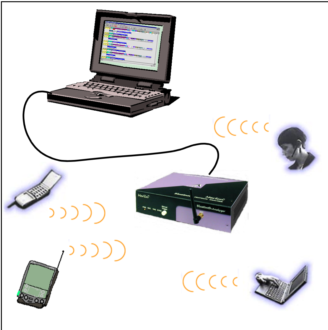
Sample Bluetooth™ Piconet with BTTracer Protocol Analyzer
