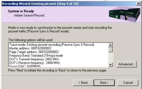
The **Advanced** button will open the Recording Options dialog box shown on page 42 and described in detail in Chapter 7.
