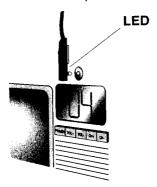
Test the *Home Producer*. The Command Center will convert the RF signal from the Home Producer into an IR signal and transmit that signal to your component through the IR signal extension cord.
