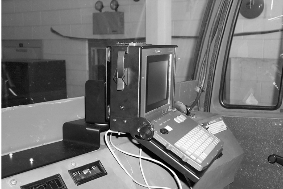
Figure 14-1 V2 computer mount (with V2 Computer installed) inside FMTV cab
