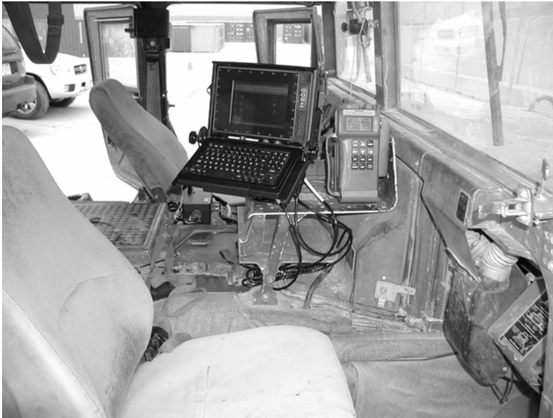
Figure 14-5 V2 Computer Mount inside HMMWV
