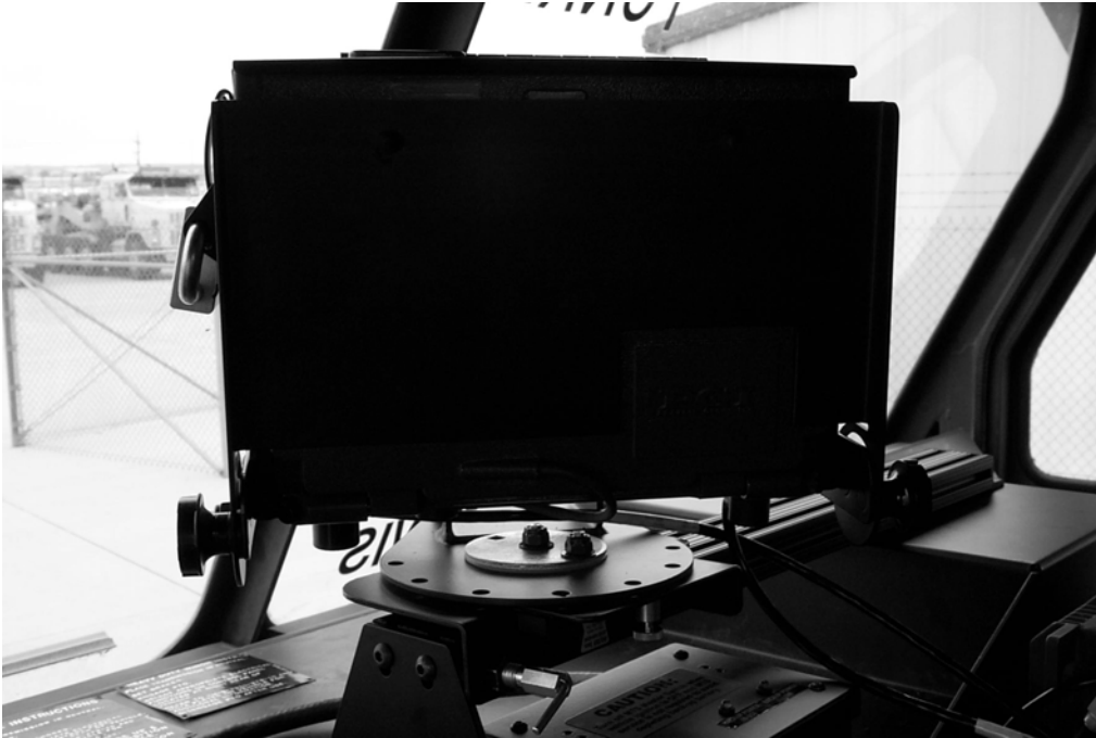
Figure 14-3 V2 computer mount (without V2 Computer) inside HEMTT cab
