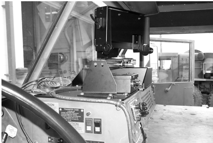
Figure 14-6 V2 Computer Mount (without V2 Computer installed) inside PLS
