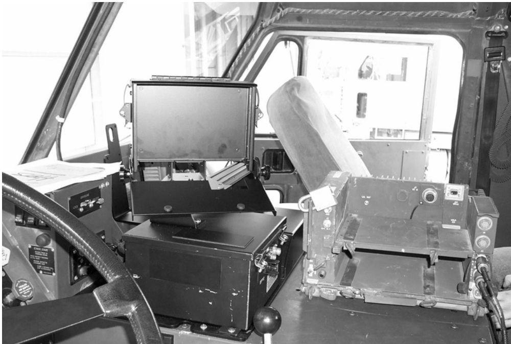
Figure 14-4 V2 computer mount (without V2 Computer installed) inside HET cab
