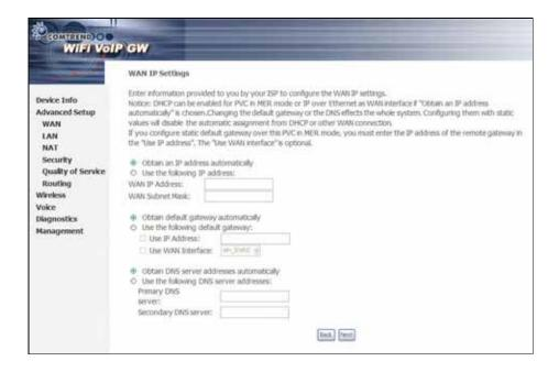
Enter information provided to you by your ISP to configure the WAN IP settings. DHCP mode must be enabled when **Obtain an IP address automatically** is chosen. Changing the default gateway or the DNS affects the whole system. Where Static mode is selected, the IP address and subnet mask must be entered, however, the **Use WAN interface** field does not need to be selected.
