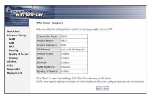
STEP 10: At this point, the device will save the configuration to flash memory and reboot. The Web UI will not respond until the device is ready. The Web UI should refresh to the default page automatically.
