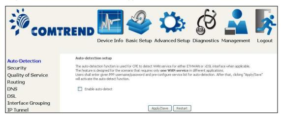
The Auto Detection page simply provides a checkbox allowing users to enable or disable the feature. Check the checkbox to display the following configuration options.
