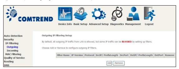
To add a filter (to block some outgoing IP traffic), click the **Add** button. On the following screen, enter your filter criteria and then click **Apply/Save**.
