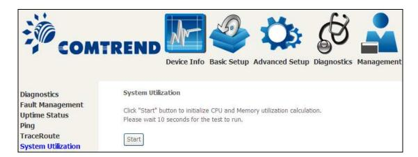
Click "Start" button to initialize CPU and Memory utilization calculation. Please wait 10 seconds for the test to run.
