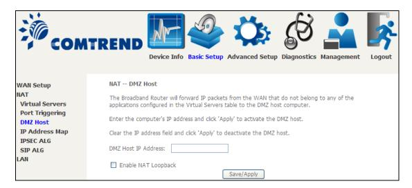
To Activate the DMZ host, enter the DMZ host IP address and click Save/Apply.
