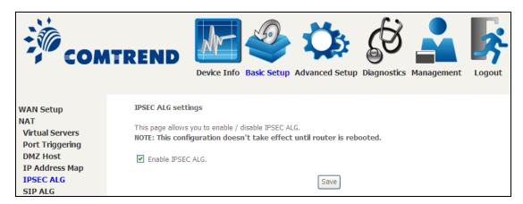
To enable IPSEC ALG, tick the checkbox and click the **Save** button.
