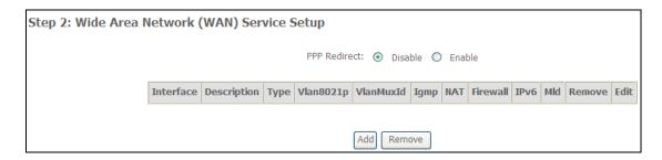
Click the **Add** button to create a new connection. For connections on ATM or ETH WAN interfaces see Appendix E - Connection Setup.
