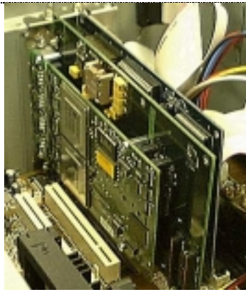
Figure 2-1 This photograph shows the SMAS board installed into a standard PCI slot.
