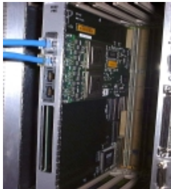
Figure 2-2 The SMAS board may be installed into a cPCI slot as shown.
