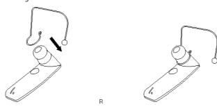
For left ear wearing, the ear hook should be inserted as shown in the diagrams.
