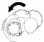
To attach the ear hook, simply insert the ear hook ring to the back of the headset gently as shown in the diagram.
