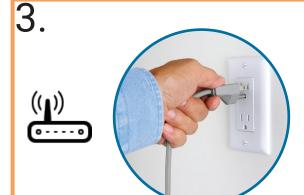
**Plug** Rently Keyless Tri-Band hub into power outlet within 20-30 feet of all smart home devices (the closer the hub, the better!).
