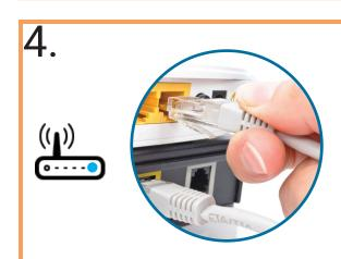
**Plug** in optional ethernet cable (if not plugged in, hub will connect via cellular). After a few minutes, light on hub will turn a solid blue. Hub is now online!
