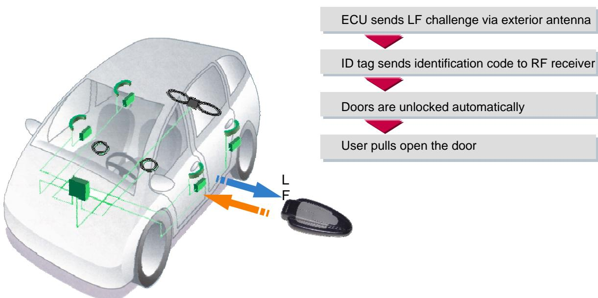
**Figure 1: Principle of Communication**
