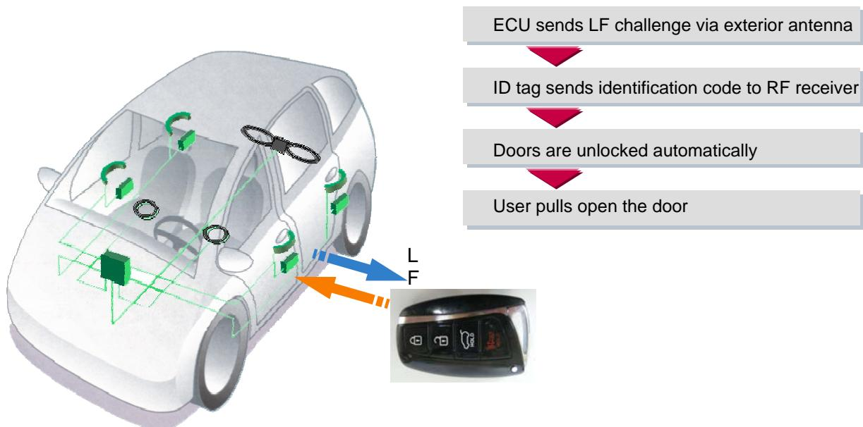
Figure 1: Principle of Communication
