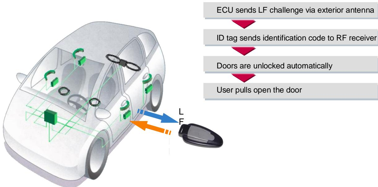
**Figure 1: Principle of Communication**
