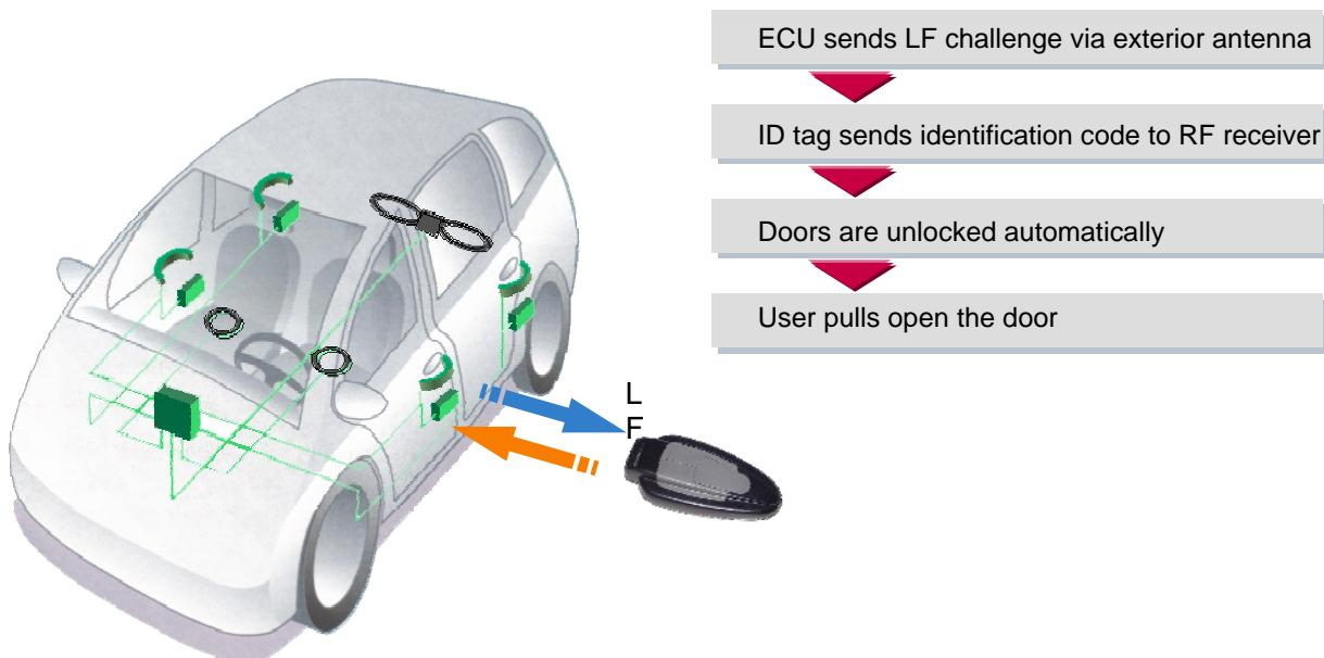
**Figure 1: Principle of Communication**
