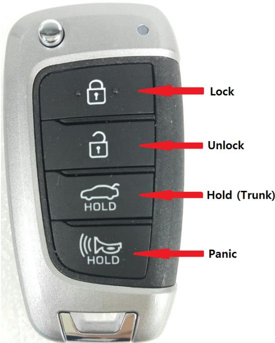
You can lock, unlock, trunk and hold your vehicle with this remote transmitter.
