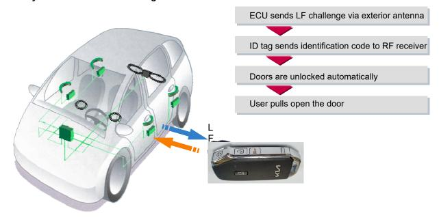
Figure 1: Principle of Communication
