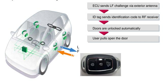
Figure 1: Principle of Communication
