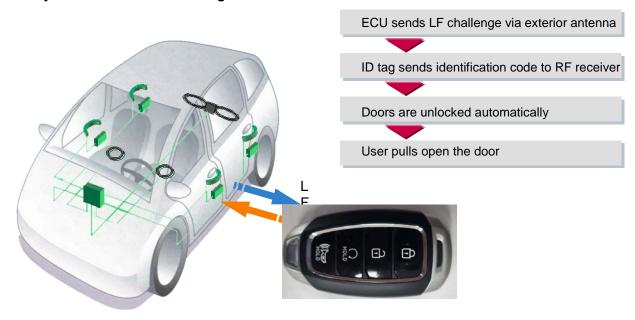
Figure 1: Principle of Communication
