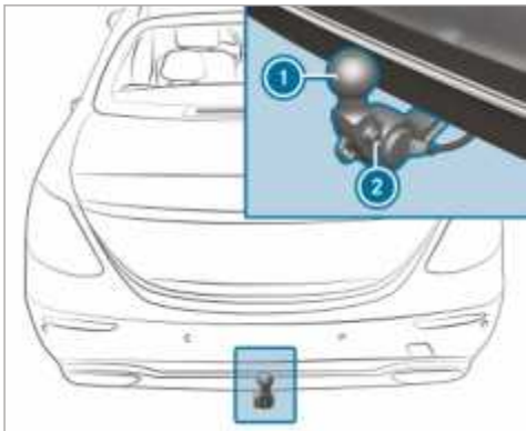
Trailer hitch (example with additional guide pins)
