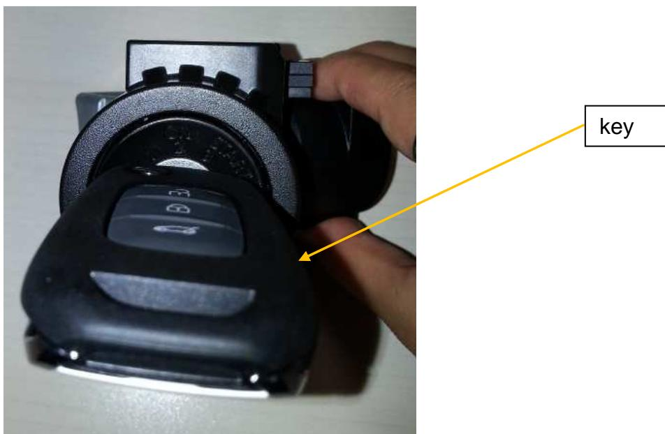
Step 2: Rotate key to start position (start letter shown on mechanical lock set). Authentication is started among key, IMMO, and EMS.
