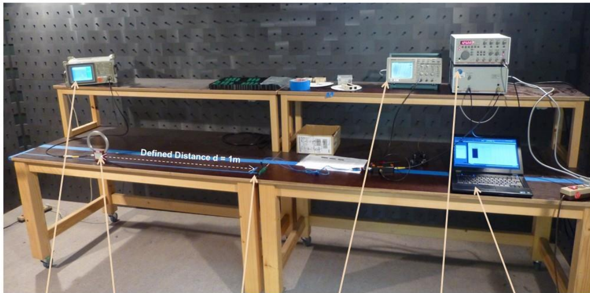
Spectrum Analyzer H-Field-Probe Transmitting ANT Transmission-Control LF-Signal-Generation Documentation
