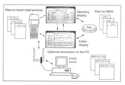
The "FILEHANDLER" program is designed so that you can use the same functions to access the files on the hand-held terminal and the files on the MDS. The directory display is available for both the hand-held terminal and the MDS. MDS files can be copied from the MDS to the hand-held terminal (and vice versa) with just a few keys.
