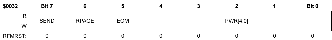
Figure 100. RFM Control Register 2 (RFCR2)
