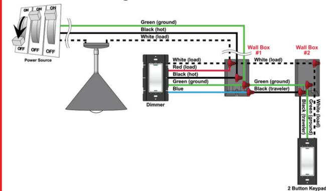
To wire the dimmer and a multi-button keypad in a two-location scenario (Control4's 3-way-switch solution) where the power is first routed to the light fixture electrical box, do the following:
