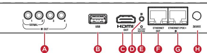
**A SERIAL and IR OUT**—3.5 mm jacks for up to four IR emitters or for a combination of IR emitters and serial devices. Ports 1 and 2 can be configured independently for serial control (for controlling receivers or disc changers) or for IR control. See "Connecting the IR ports/serial ports" in this document for more information.
