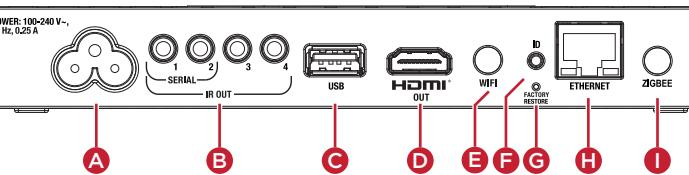
**A Power port**—AC power connector for an IEC 60320-C5 power cord.
