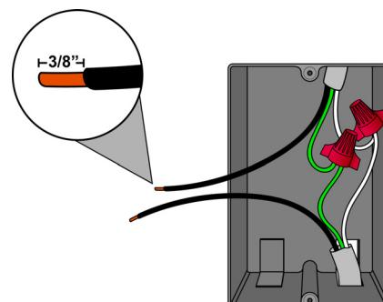
**IMPORTANT:** The National Electric Code (NEC) requires 6 inches of extended wire from the wall box. If your wiring does not meet this requirement, you will not meet code. Do NOT cut wire shorter than 6 inches.
