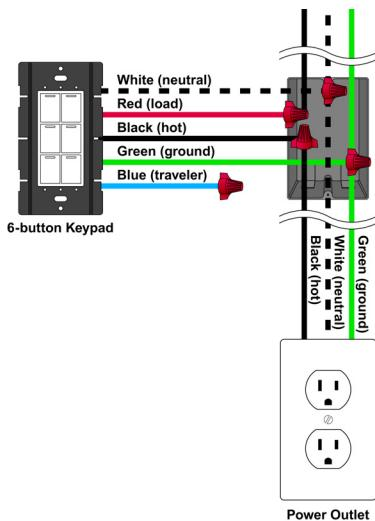
To wire the 6-button keypad for a Control4 single-switch environment with the power coming from a nearby power outlet or light switch, connect and cap with a wire nut the wires indicated in the table.
