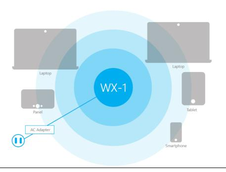
The WX-1x can be configured in several modes: Access Point, WDS Root Access Point, WDS Repeater or WDS Bridge. When shipped from the factory, the WX-1x is set to Access Point mode. The default IP address of the WX-1x is **192.168.1.250** and username/password of **pakedge/pakedgea**.
