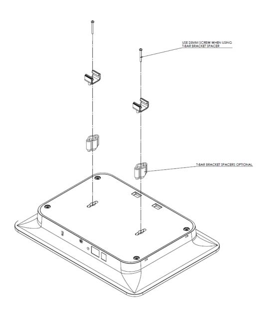
2. Line up the T-bar brackets with the T-Bar. Press down until the T-bar brackets snap on.
