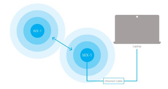
• **WDS Repeater** – The repeater also receives wireless signal from another access point. However, unlike a brige access point, a repeater access point sends out Wi-Fi so that client devices can connect to it wirelessly.
