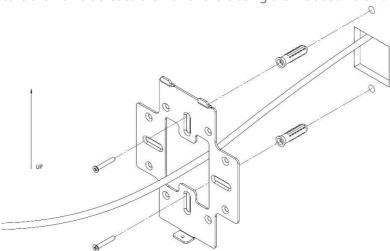
**Horizontal mount**: Line up the slots and secure the wall bracket to the wall anchors using the included hardware.
