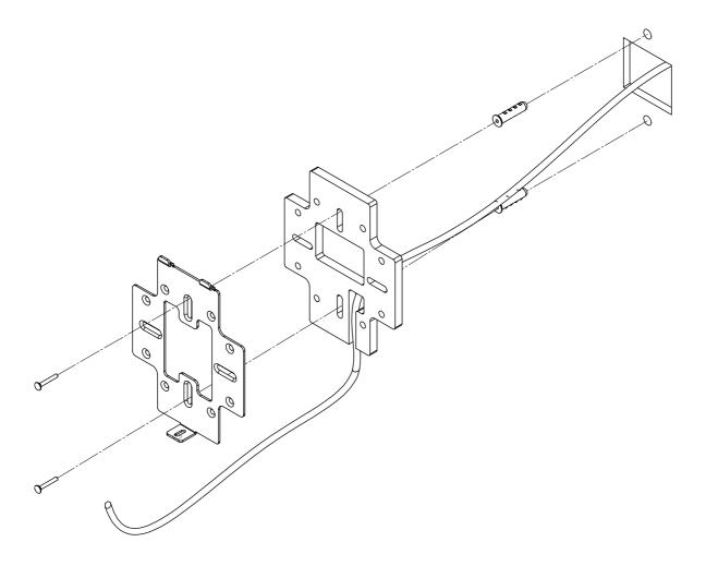
Line the two tabs on the top of the wall bracket with the two pockets on the back of the access point. Slide the WAP downwards to lock it in place and secure with security screw.
