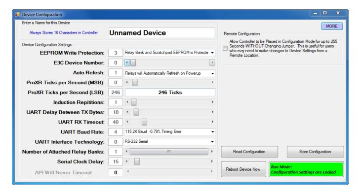
**NOTE:** NCD Devices must be in Configuration mode to make changes. Use the green button shown above to change to Configuration mode. You may also use the Program/Run-jumper to change modes. NEVER leave the jumper in Program mode. Program mode is for configuration changes only. Use RUN mode for daily operation.
