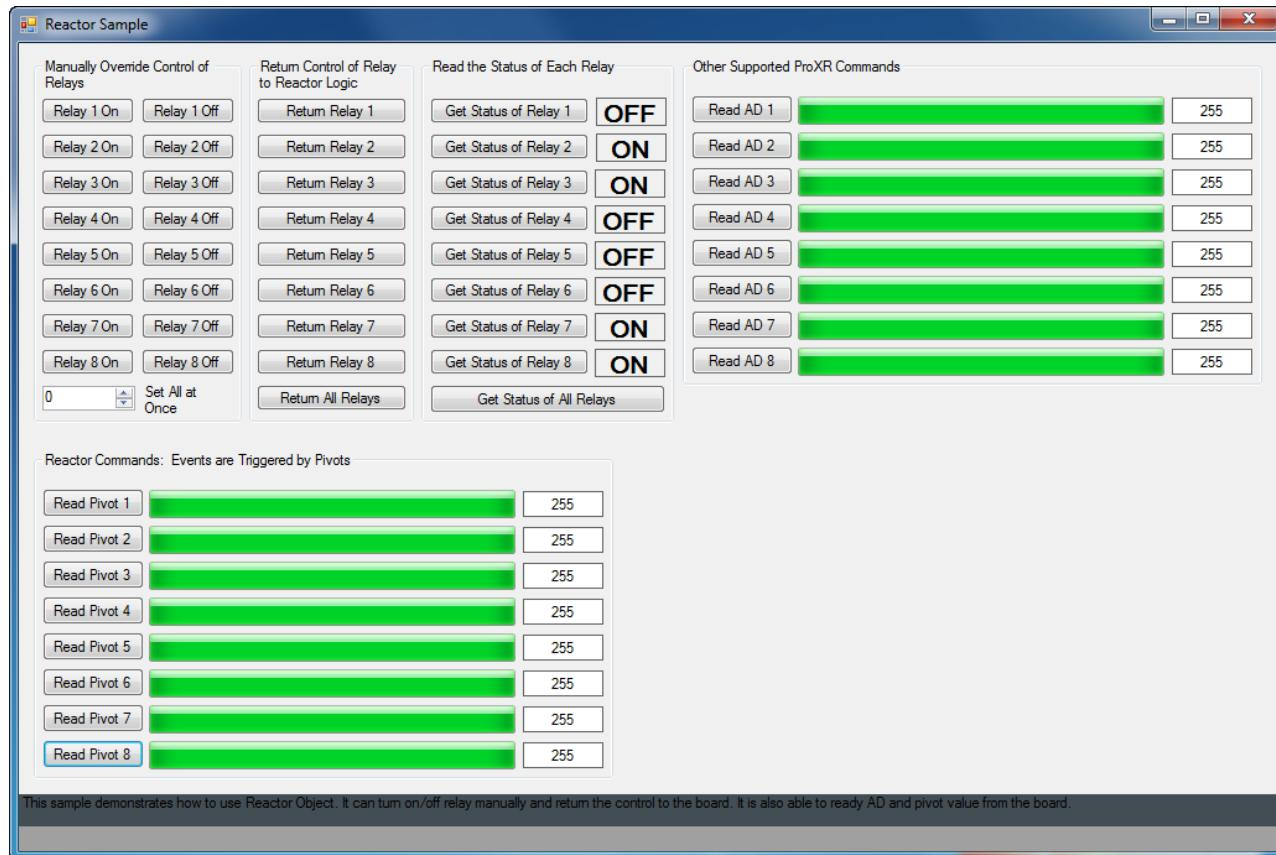
Set and Receive Relay Status and Read AD Input values for all Reactor Series Controllers.
