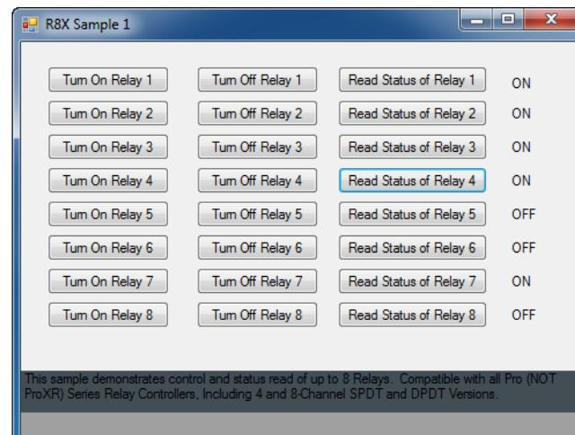
This sample demonstrates control and status read of up to 8 Relays. Compatible with all Pro (NOT ProXR) Series Relay Controllers, including 4 and 8-Channel SPDT and DPDT Versions
