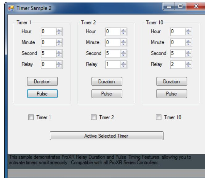
This sample demonstrates ProXR Relay Duration and Pulse Timing Features, allowing you to activate timers simultaneously. Compatible with all ProXR Series Controllers,
