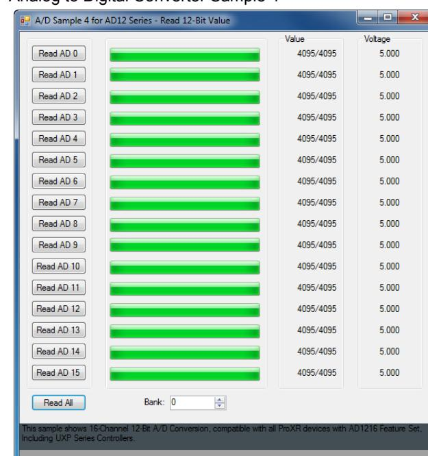
This sample shows 16-Channel 12-Bit A/D Conversion, compatible with all ProXR devices with AD1216 Feature Set, including UXP Series Controllers.
