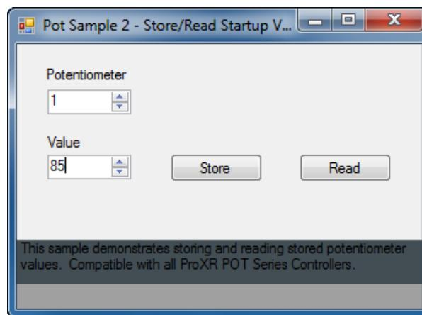
This sample demonstrates storing and reading stored potentiometer values. Compatible with all ProXR POT Series Controllers.
