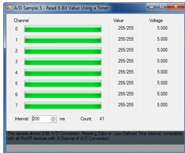
This sample shows 8-Bit A/D Conversion, Reading data on User-defined Time Interval, compatible with all ProXR devices with 8-Channels of A/D Conversion.
