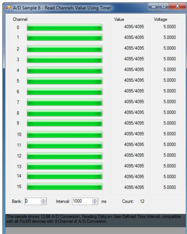
This sample shows 12-Bit A/D Conversion, reading data on User-defined Time Interval, compatible with all ProXR devices with 8-Channels of A/D Conversion.
