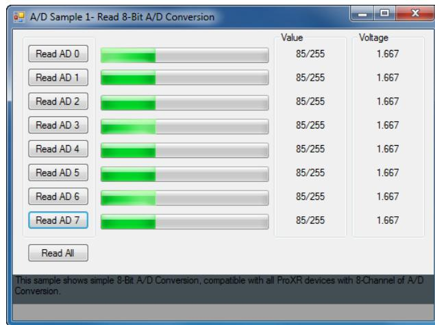
This sample shows simple 8-Bit A/D Conversion, compatible with all ProXR devices with 8-Channels of A/D Conversion.
