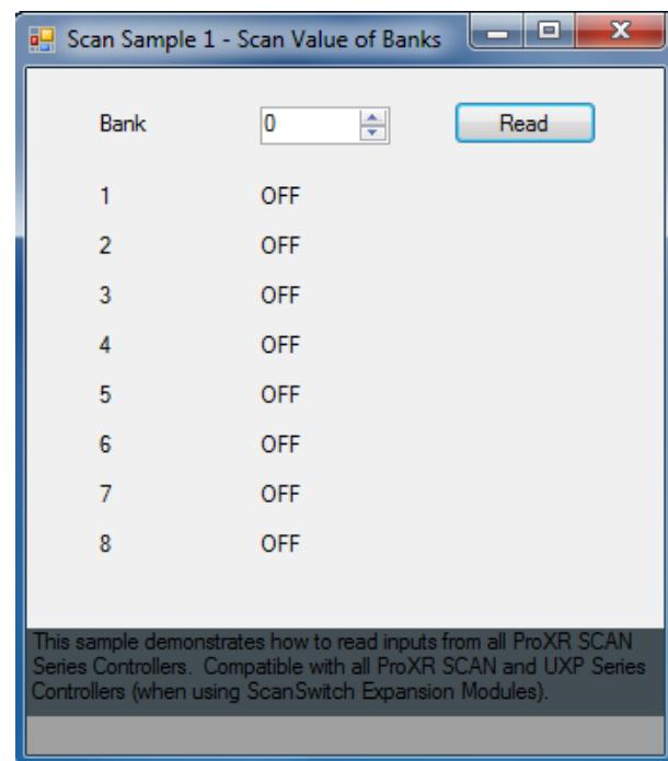
This sample demonstrates how to read inputs from all ProXR SCAN Series Controllers. Compatible with all ProXR SCAN and UXP Series Controllers (when using ScanSwitch Expansion Modules).
