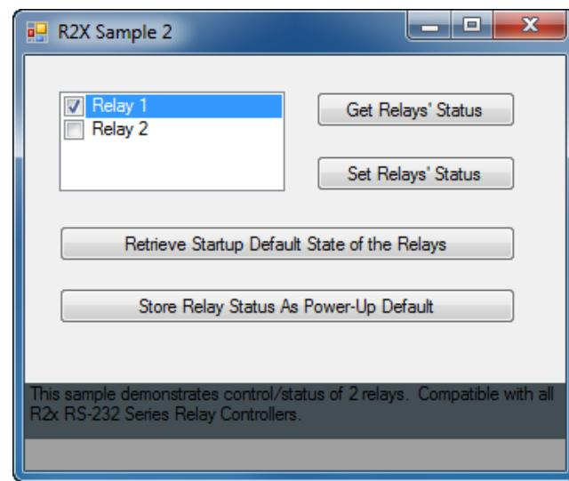
This sample demonstrates control/status of 2 relays and demonstrates data storage features . Compatible with all R2x RS-232 Series Relay Controllers.
