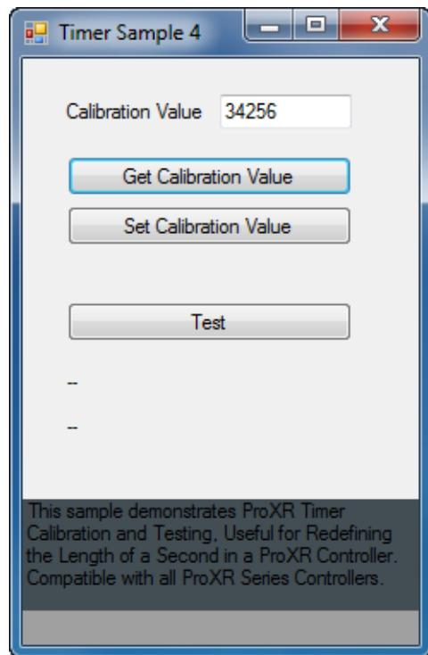
This sample demonstrates ProXR Timer Calibration and Testing, Useful for Redefining the Length of a Second in a ProXR Controller. Compatible with all ProXR Series Controllers.
