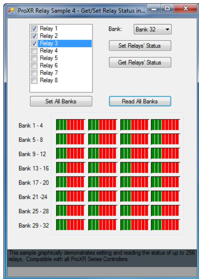
This sample graphically demonstrates setting and reading the status of up to 256 Relays. Compatible with all ProXR Series Controllers.
