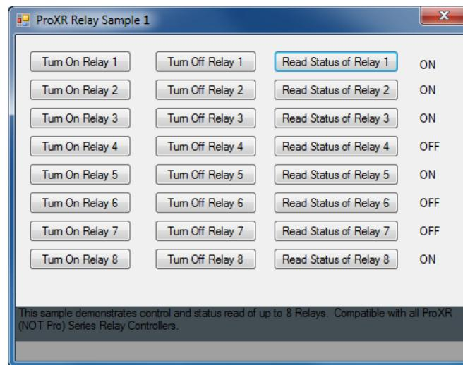
This sample demonstrates control and status read of up to 8 relays. Compatible with all ProXR (Not Pro) Series Relay Controllers.
