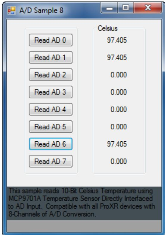
This sample reads 10-Bit Celsius Temperature using MC9701A Temperature Sensor directly interfaced to AD Input. Compatible with all ProXR devices with 8-Channels of A/D Conversion.
