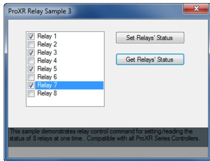
This sample demonstrates relay control command for setting/reading the status of 8 relays at one time. Compatible with all ProXR Series Controllers.
