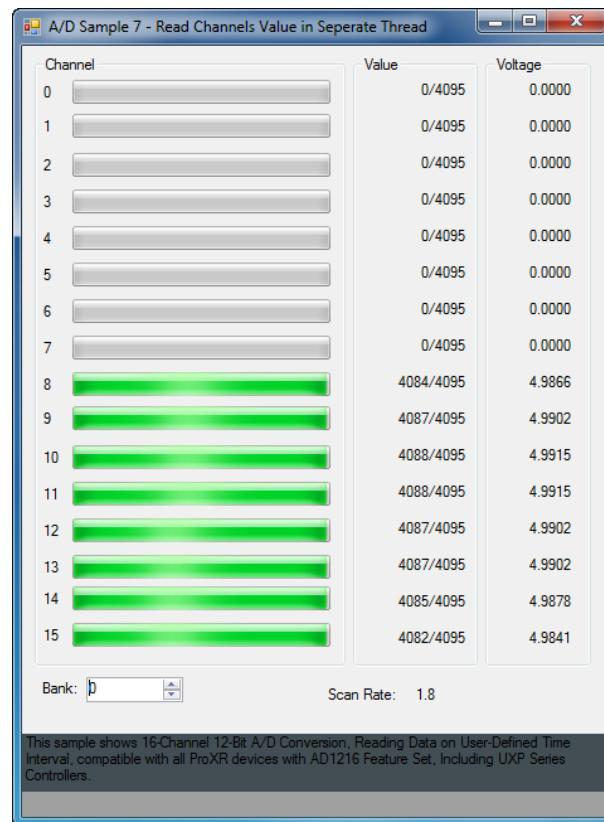
This sample shows 16-Channel 12-Bit A/D Conversion, reading data on User-defined Time Interval, compatible with all ProXR devices with AD1216 Feature Set, including UXP Series Controllers.
