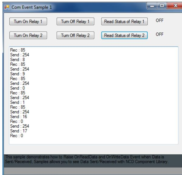
This sample demonstrates how to Raise OnReadData and OnWriteData Event when data is Sent/Received, samples allows you to see data Sent/Received with NCD Component Library.
