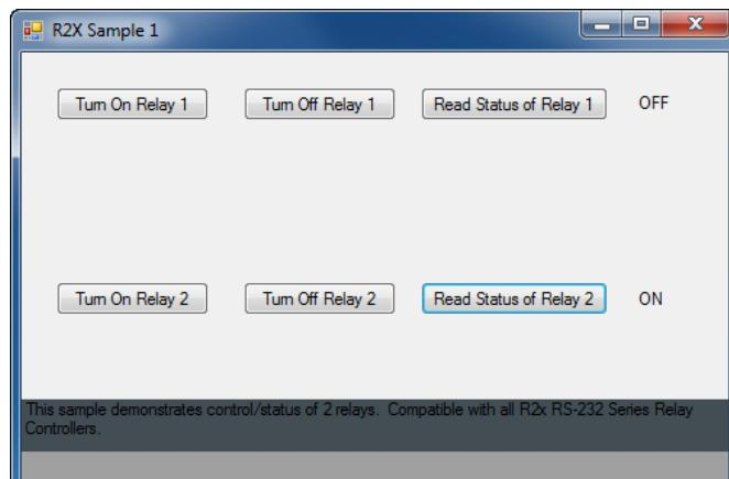
This sample demonstrates control/status of 2 relays. Compatible with all R2x RS-232 Series Relay Controllers.
