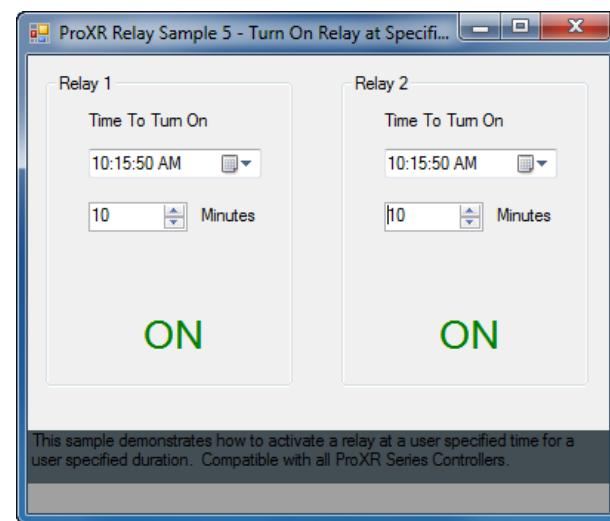
This sample demonstrates how to activate a relay at a user specified time for a user specified duration. Compatible with all ProXR Series Controllers.
