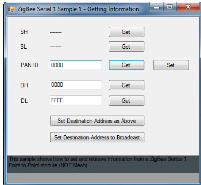
This sample shows how to send and retrieve information from a 802.15.4 Wireless Series 1 Point to Point module (NOT Mesh).
