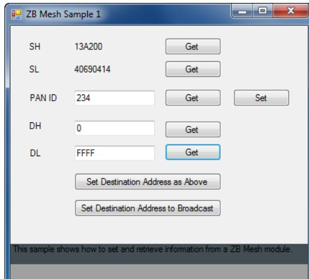
This sample shows how to set and retrieve information from a ZigBee module.
