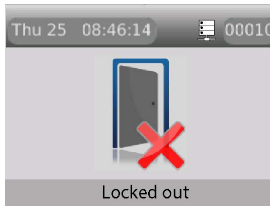
Figure 60 Interlock locked out display message in door mode
