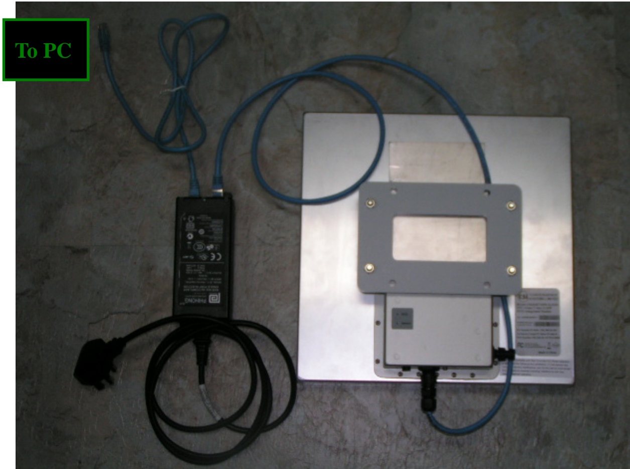
Figure 2-5 POE adaptor Setup
