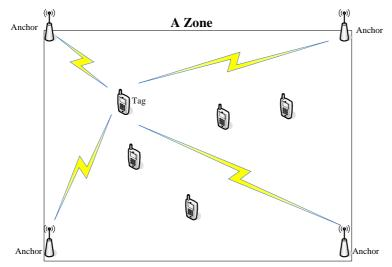
In a minimum system, 4 anchors -3 slave anchors CS5111TD/CS5112TD and 1 master anchor CS5113TD/CS5114TD- are installed in a zone. However, the more the anchors are installed, the higher the accuracy of the tag position to be obtained. The accuracy of positioning is +/-1 meter.
