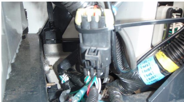
Interface Plug connected to Serial Port on Reefer
