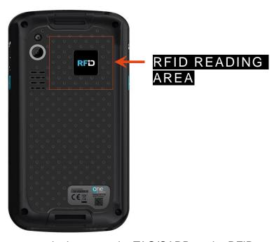
C-One<sup>2</sup> LF AGRIDENT with RFID options to read, please put the TAG/CARD on the RFID area.
