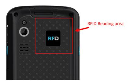
For C-One<sup>2</sup> LF AGRIDENT with RFID option, to read put the TAG/CARD on the RFID area.
