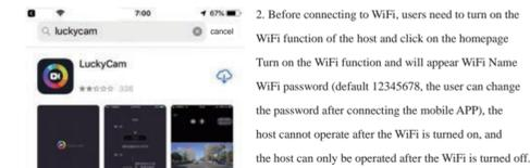
2. Before connecting to WiFi, users need to turn on the WiFi function of the host and click on the homepage WiFi function and will appear WiFi Name WiFi password (default 12345678, the user can change the password after connecting the mobile APP), the host cannot operate after the WiFi is turned on, and the host can only be operated after the WiFi is turned off.
