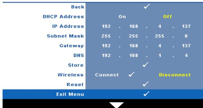
**DHCP ADDRESS**—If a DHCP server exists in the network to which the projector is connected, the IP address will automatically be acquired when you select DHCP **On**. If DHCP is **Off**, manually set the IP Address, Subnet Mask, and Gateway. Use   to select the number of IP Address, Subnet Mask, and Gateway. Key in Enter to confirm each number and then use   to set the next item.
