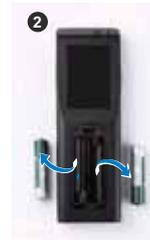
3 Insert the batteries and align their polarity correctly according to the marking in the battery compartment.
