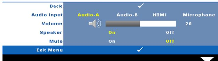
**AUDIO INPUT**—Select the Audio input source, options are: Audio-A, Audio-B, HDMI and Microphone.
