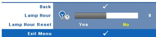
**LAMP HOUR**—Displays the operating hours since the last lamp timer reset.
