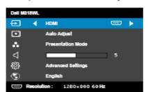
**HDMI** — Press ⊘ to detect a HDMI signal.
