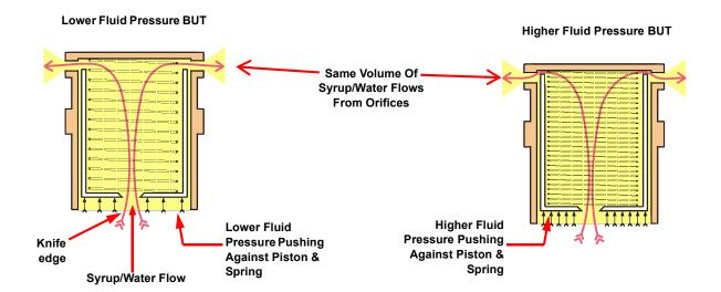
The position of the piston inside the sleeve is determined by the upward pressure of the liquid against the base of the piston and the downward pressure of the spring inside the piston (not shown here). The pressure of the spring is regulated by the adjusting screw.
