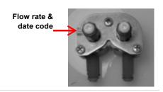
13. To disassemble the flow control: Remove screws and pull retainer forward. Remove top flow control subassemblies exposing flow controls.
