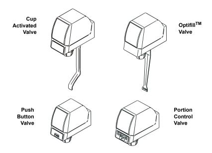
The UF-1 and UFB-1 valves are the same as described above with minor differences for juice applications. In the UF-1 and UFB-1 valve concentrate enters the nozzle assembly higher providing a better mix of concentrate and water in the cup. In addition, the orifices for concentrate are larger to avoid clogging. The concentrate diffuser is gray allowing for easy identification.
