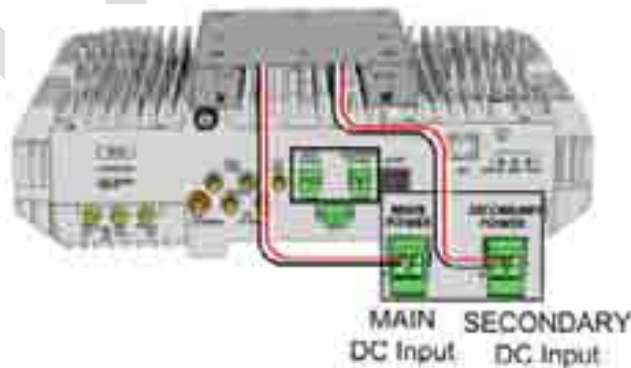
Figure 5-94. RAU5 MAIN and SECONDARY DC Input Connections
