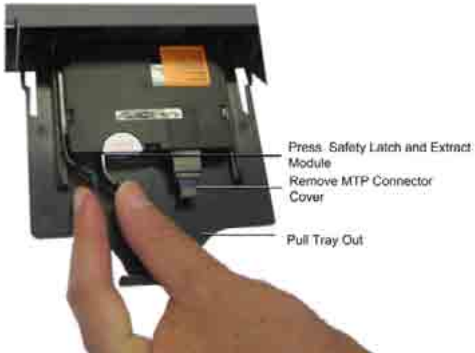
Figure 5-61. Extracting Edge Module
