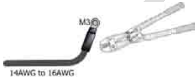
Figure 5-17. Crimping the Terminal Rings onto the DC Wire
