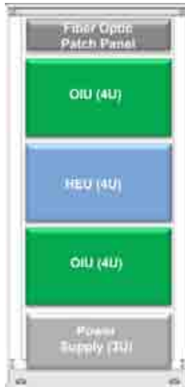
Figure 4-1. Example of Communication Rack Installation
