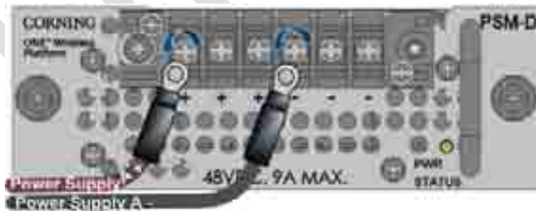
Figure 5-18. Connecting PSM-DC Wire Pairs
