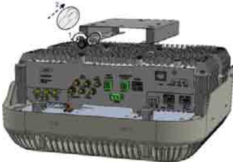
Figure 10-2 Removing Bracket and Antenna Skirt
