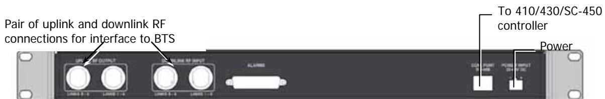
Figure 11. BU Rear Panel (RF Connections)
