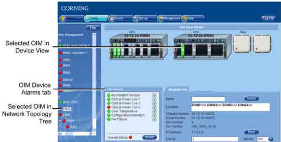
Figure 9-9. OIM Alarms Tab and Device View
