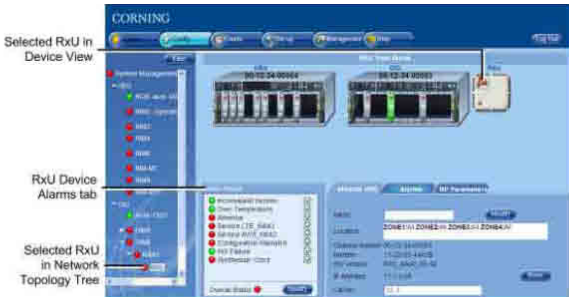
Figure 9-13. RxU Alarms Tab and Device View
