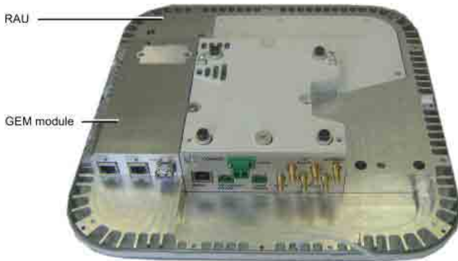
Figure 5-2. Inserting GEM in the RAU Enclosure
