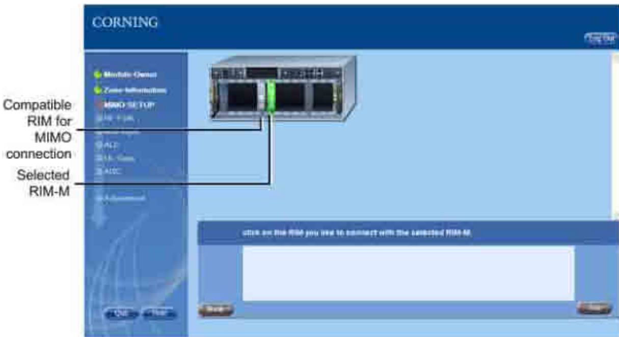
Figure 6-20. MIMO Setup Phase
