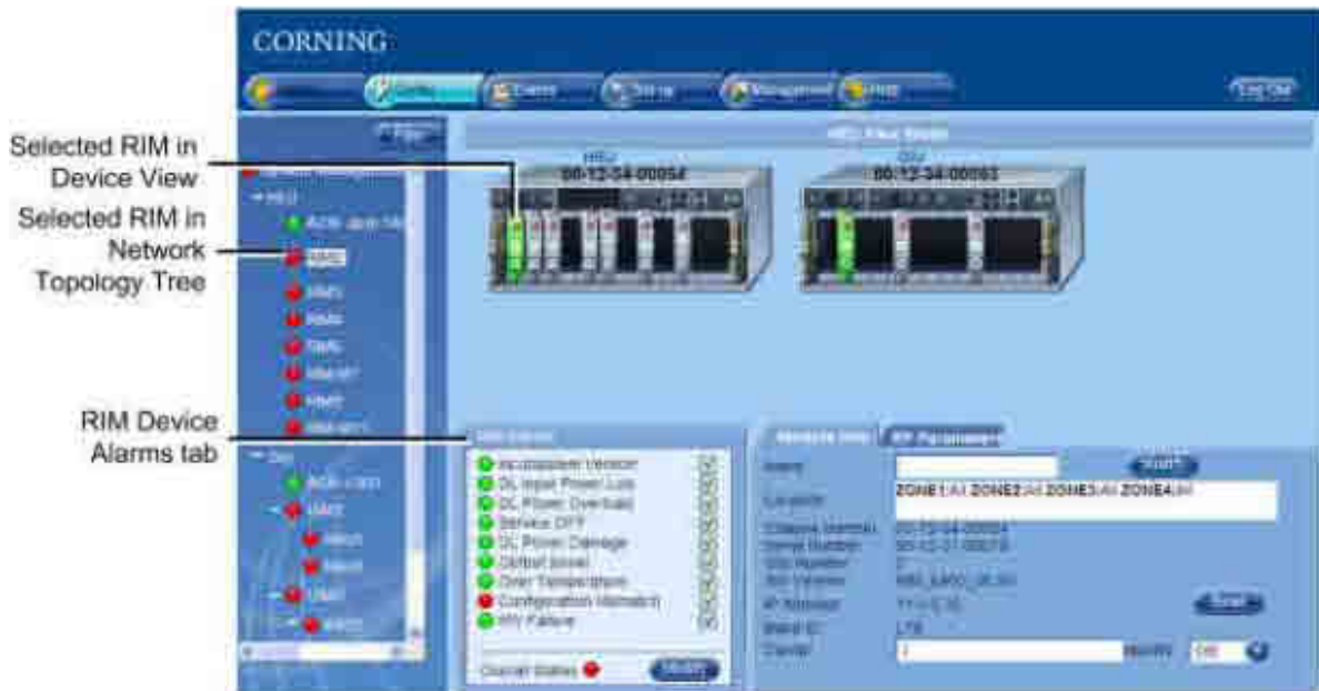
Figure 9-7. RIM Device View and Alarms
