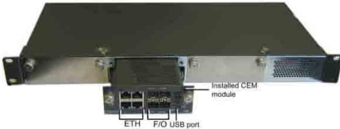
Figure 3-4. CEM Interfaces (Installed in CEU)
