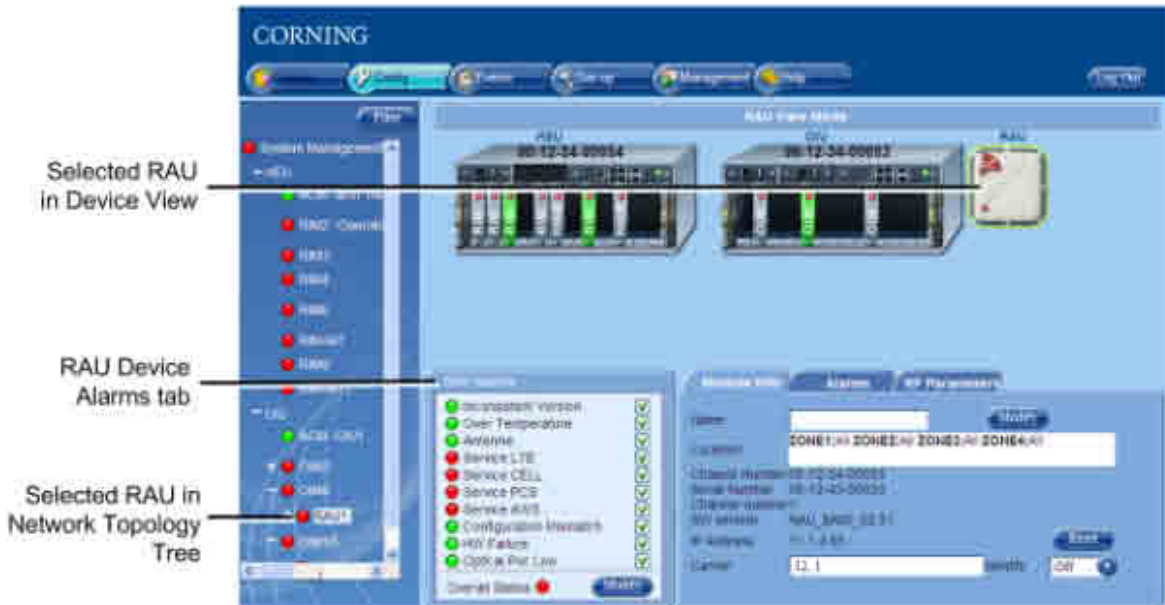
Figure 9-11. RAU Alarms Tab and Device View Mode
