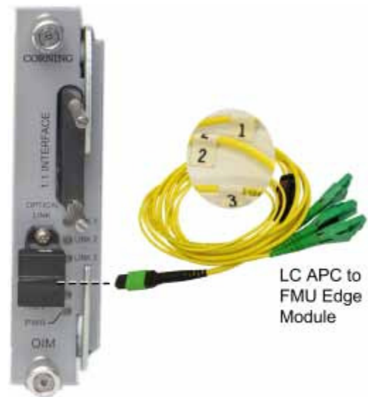
Figure 4-21. OIM Fiber Connections
