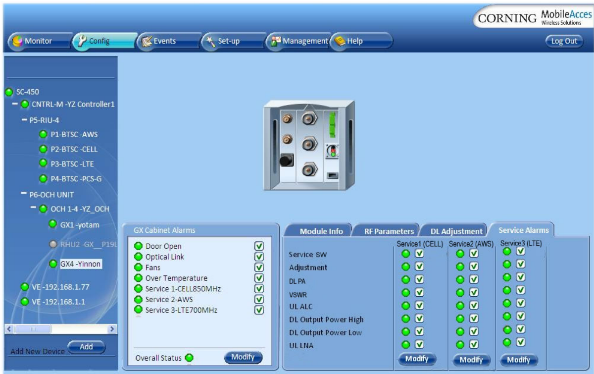
Figure 4-3. GX Service Alarms Tab
