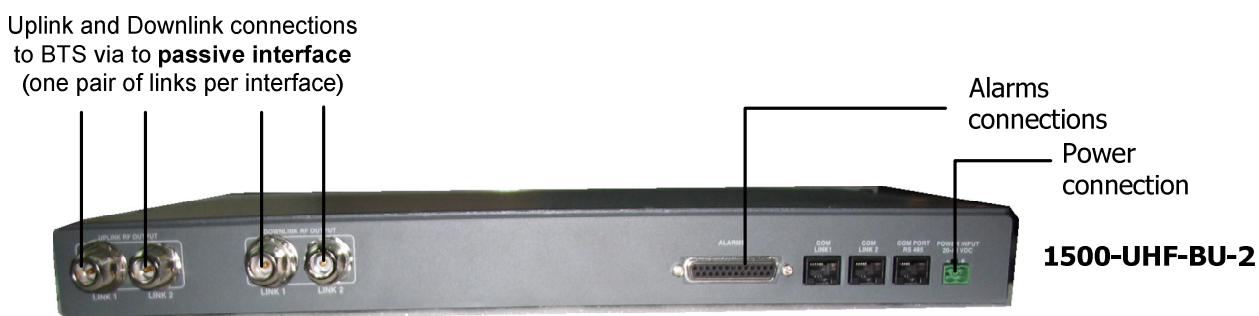
Figure 3-2: 1500-UHF-BU-2 Building Connections
