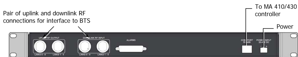
Figure 11. MA BU Rear Panel (RF Connections)
