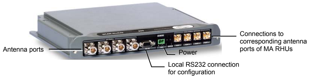
Figure 2-1. MobileAccess 850 Front Panel View
