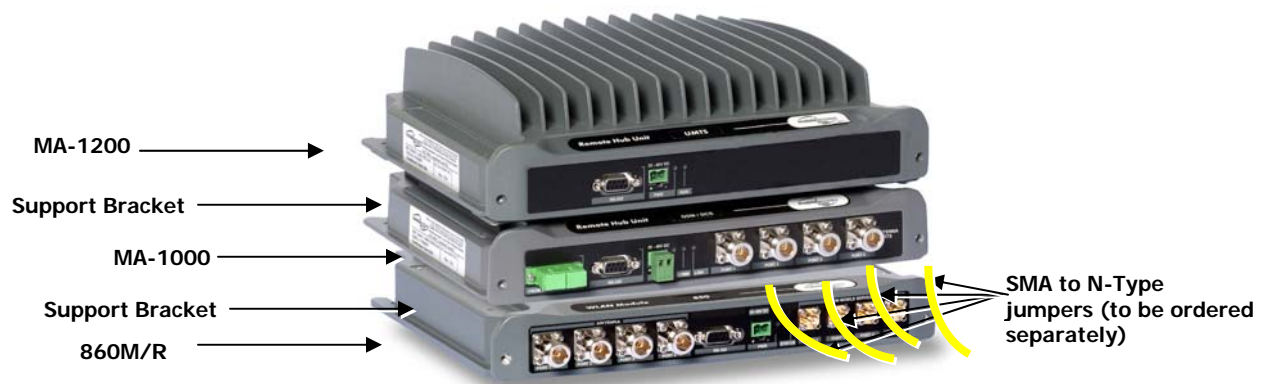
Figure 3–9: 860M/R, MA-1200 and MA-1000 Assembly (Scenario A)
