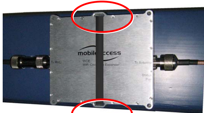
Figure 3-2: WCE Mounting with Tie Fixture
