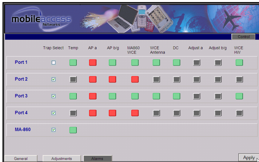
Figure 4–4: 860M/R GUI Control Screen – Alarms Tab
